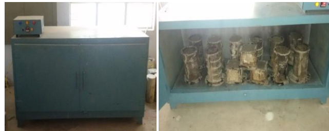
Fig 2: Specimens were kept in Oven for curing
