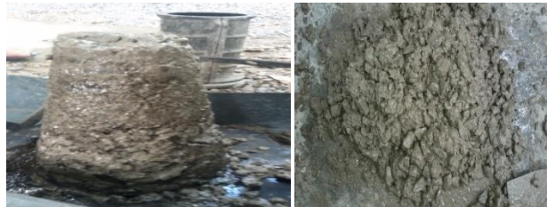
Fig 1: Slump cone test of Geopolymer Concrete for workability
